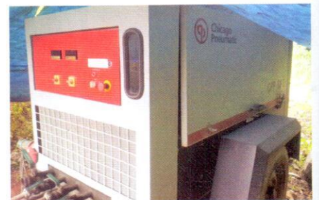
The Chicago Pneumatic compressor is being used to power drilling equipment at the quarry
