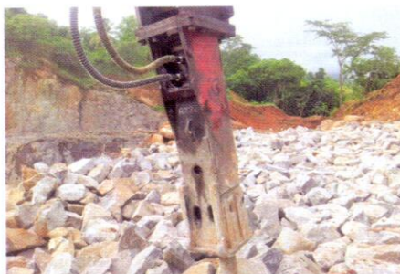
Based in Kerala, India, National granite is using Chicago Pneumatic hydraulic hammers for secondary breaking of its granite production
